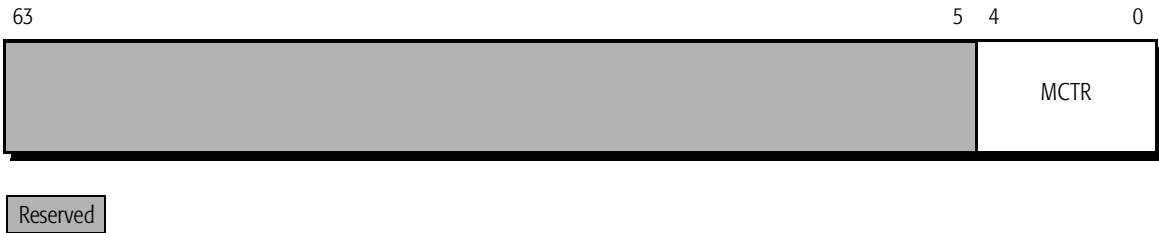
Figure 31. Machine-Check Type Register (MCTR)
